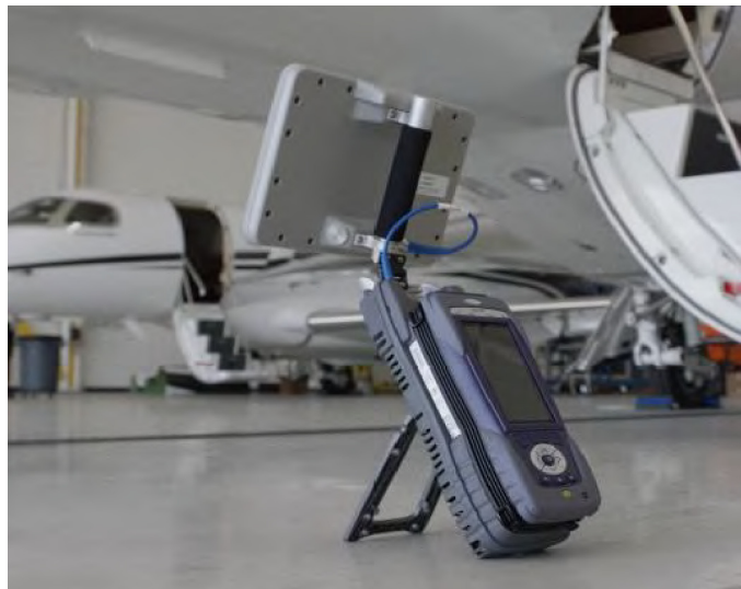
Figure 3-2 Over-the-Air Test Set-Up
