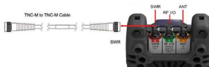
Figure 10-2 VSWR Calibration RF Port Setup
