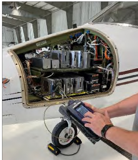
Figure 3-5 Direct to UUT Test Setup
