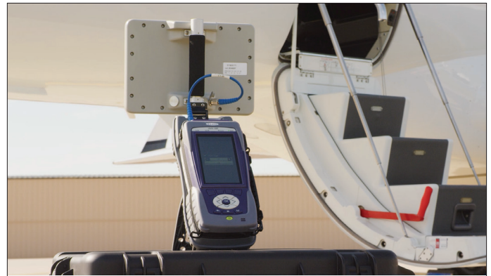
The AVX-10K operates the same as the IFR6000/6015 when performing the Far 43 and 43 MOD test.
