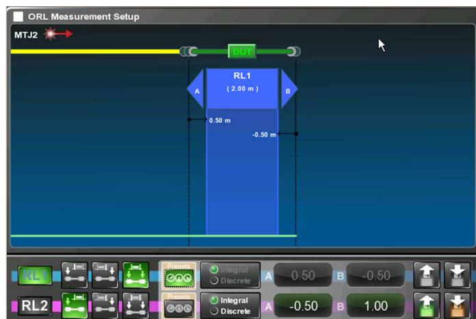
Figure 9: ORL setup screen for Integral Mode measurement.
