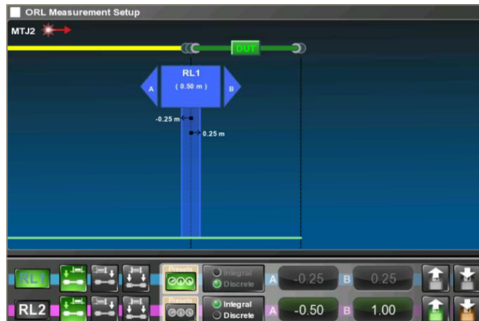
Figure 8: ORL set-up screen for an optical connector measurement
